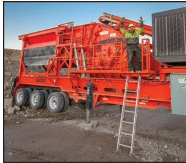
Crosby Excavating's Eagle 1200-25 closed-circuit crusher/screener processes up to 300 tons per hour while reducing the company's fuel costs. The 1200 also removes rebar and produces two products that meet INDOT specifications.
