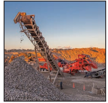
Crosby Excavating's Eagle 1200-25 closed-circuit crusher/screener processes up to 300 tons per hour while reducing the company's fuel costs. The 1200 also removes rebar and produces two products that meet INDOT specifications.
