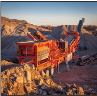
Crosby Excavating's Eagle 1200-25 closed-circuit crusher/screener processes up to 300 tons per hour while reducing the company's fuel costs. The 1200 also removes rebar and produces two products that meet INDOT specifications.
