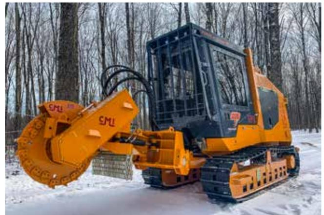
The new S175 will also fit older C175 models since the three-point mount plate is the same. That said, CMI highly recommends contacting your local dealer regarding installation to determine whether in-line, flow-control valves are required to slow down the speed of certain functions such as swing cylinders and tilt down.
