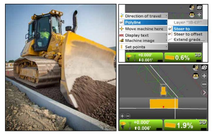
On any given building pad in a design file, a dozer operator may want to extend the grade of the pad. Why? One good example is so other equipment that will be working on/around the building pad later has a nice, level surface on which to work. An excavator coming in after the dozer to dig footers for a building will be able to move around the designed building pad more quickly and efficiently because of an even surface surrounding the area.
