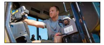
PDC, they can finetune the automatics' blade control. "An operator can push the blade to go deeper, for instance, and the machine will remember—it will maintain the automatics but cut more through the push," Fenster said. In iMC machines without PDC, the machine only maintains the change as long as the operator holds the lever.
