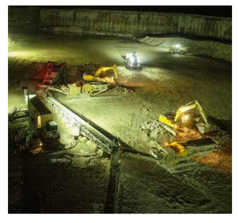
The main crusher—a 3862 track jaw crusher had a bearing failure this summer. The company needed a fill-in replacement while the machine was being repaired, and Columbus Equipment Company was able to supply two machines—an FT4250 horizontal impact crusher and an FT2650 jaw crusher—both tracked, portable machines.
