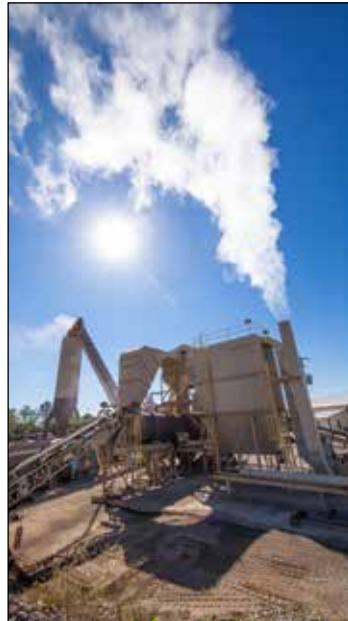
WA320 Operator Carl Lowry (left) keeps a hungry G&J Paving plant fed with gravel, sand and RAP. The gravel dryer sucks up 3,000 gallons of used motor oil/day, burning at over 1,000°. Ultimately, around 1,200 tons of HMA (right) head into the 10"-thick tower—at around 380°—every day.
